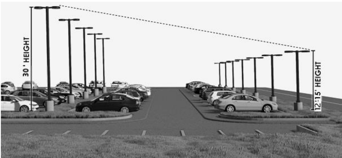
Figure 5.7.4. Parking Area Lighting Standards Illustrative Example
