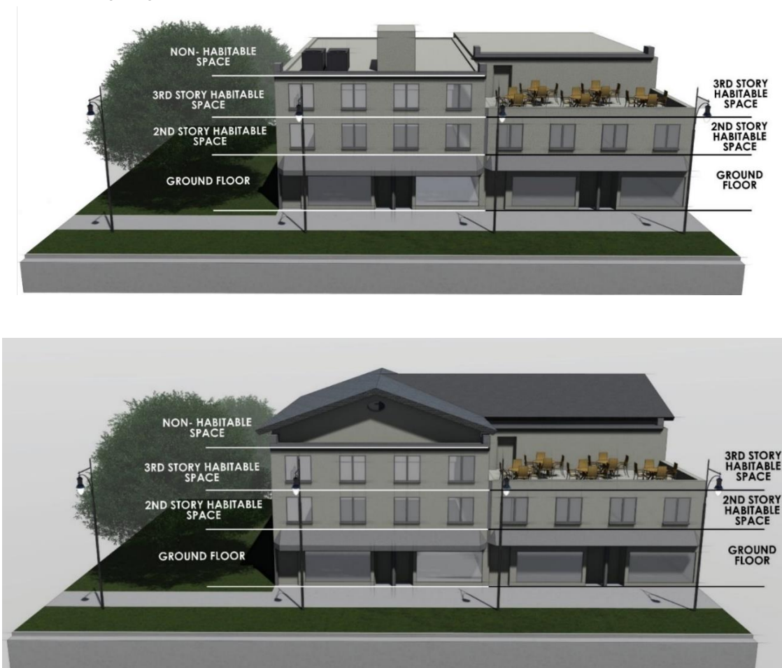
Figure 5.1.1. Building Height Illustrations
